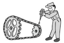
③ Conveyor chains and sprockets are consumable parts. As such, they require proper periodic maintenance and replacement. Avoid replacing only part of a chain. Replace the chain as a whole.
